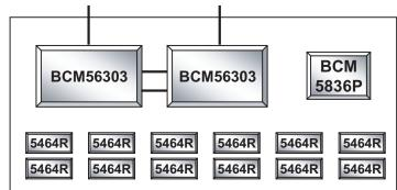
The BCM56303 is the fifth generation of the highly-integrated and costeffective Broadcom StrataSwitch and StrataXGS product line in a singlechip solution with 24 GbE ports and three 10-GbE/HiGig+ uplink ports. The BCM56303 is a member of the Value GbE product line, with a corresponding pin-compatible member in the Feature GbE product line—BCM56503. The BCM56303 incorporates 24 GbE ports that can operate 10/100/1000 Mbps. The uplink ports can operate in two modes:
